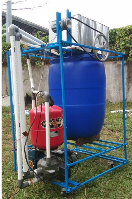
Gambar 4.12. Assembling Hardware Mekanik PLTA
