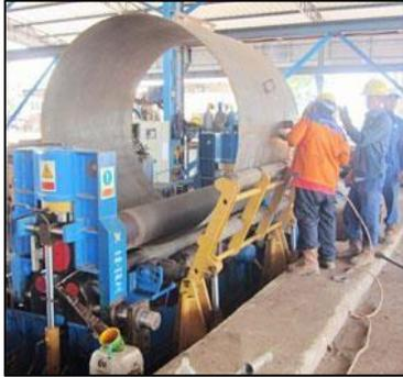
Gambar 1.17 *Plate Rolling Machine*
