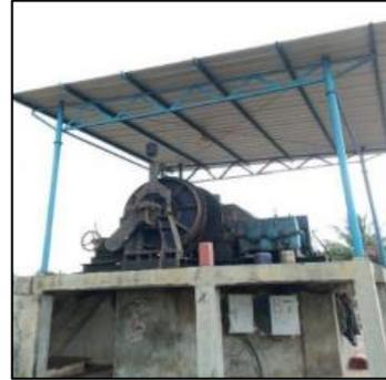
Gambar 1.18 *Winch Slipway*
