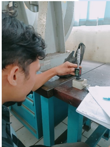
Gambar 4. 8 Prosedur Uji Kekerasan
