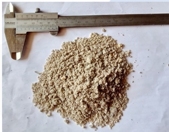
Gambar 3. 4 Boiler Fly Ash.
