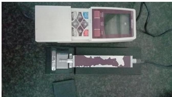
Gambar 3. 16 Proses Kalibrasi *Surface Roughness Tester*
