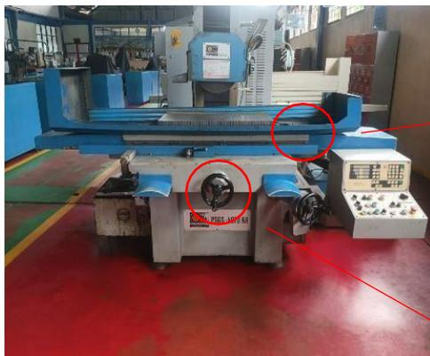
*Gambar 1. 2 Mesin Gerinda Datar Reform PSGS-4070 AH*
