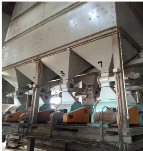
Gambar 2.19 *Ripple Mill*
