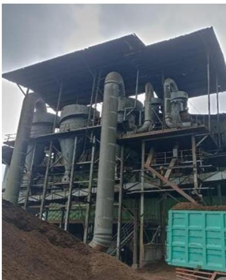
*Gambar 2.16 Fibre Cyclone*
