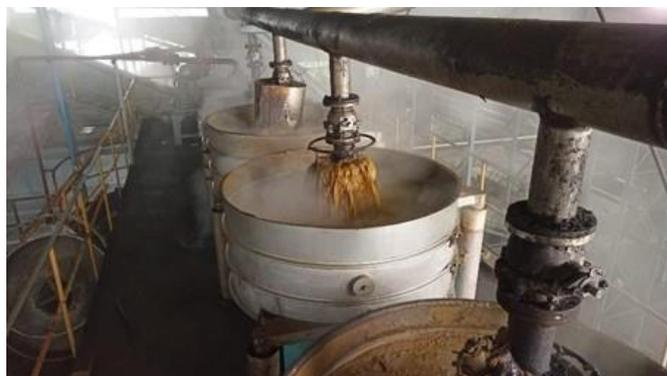
*Gambar 2.10 Vibrating Sludge*
