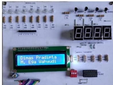
Gambar 4. 17 *Output* Mikrokontroler LCD 2 x 16
