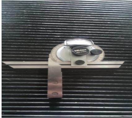
Gambar 4.11 *Bevel Protractor*
