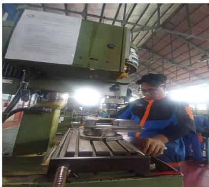
Gambar 4.24 Proses *Milling*
