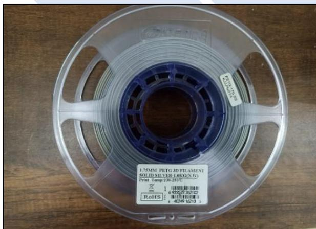
Gambar 3.8 Filament PETG (*Polyethylene Terephthalate Glycol*)
