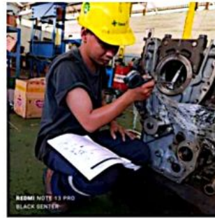
Gambar 18 Proses pengukuran main cup bearing
