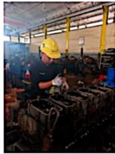
Gambar 17 Proses Overhoull Mesin Yanmar 6AYM-WST
