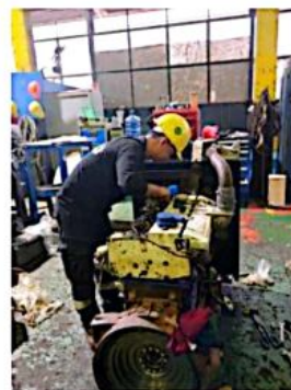
Gambar 20 Proses overhoull Genset Perkins
