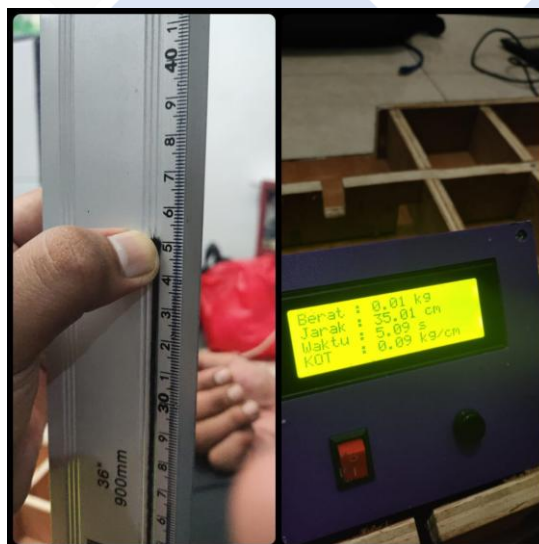
Gambar 4. 32 Hasil Pengujian Sensor Rotary Encoder
