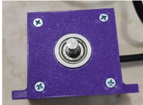
Gambar 4. 24 Pelindung Sensor Rotary Encoder 3D Printing
