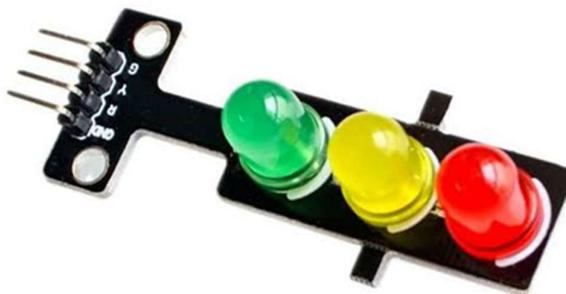
*Gambar 2. 8 Mini Traffic Light Display Module*
