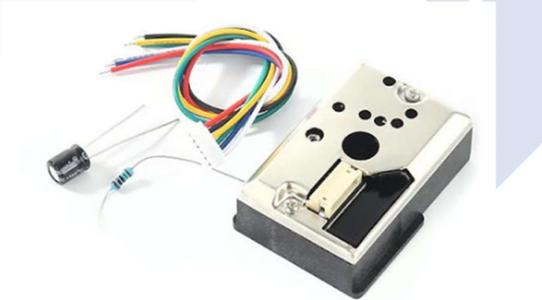
*Gambar 2. 5 Debu Sensor GP2Y1010AU0F*
