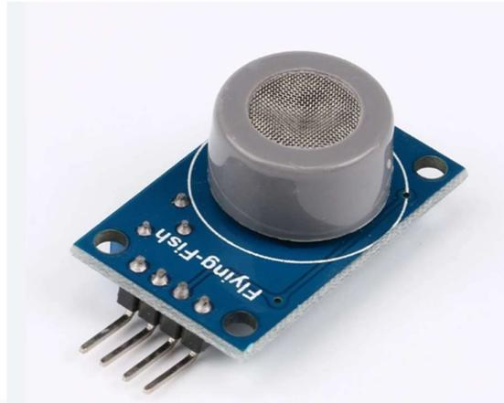
Gambar 2. 4 Sensor Gas MQ-7
