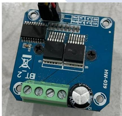
Gambar 2.8 Driver Motor IBT-2 BTS7960
