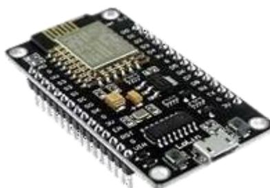
Gambar 2.6 NodeMCU ESP8266
