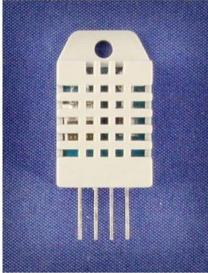
Capacitive-type humidity and temperature module/sensor
