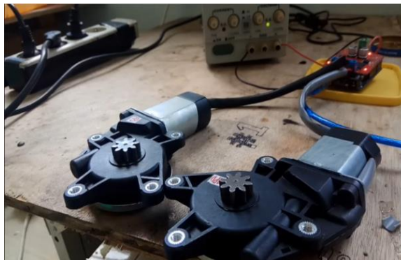
Gambar 4. 35 Pengujian Driver IBT-02 Terhadap Motor DC Power Window
