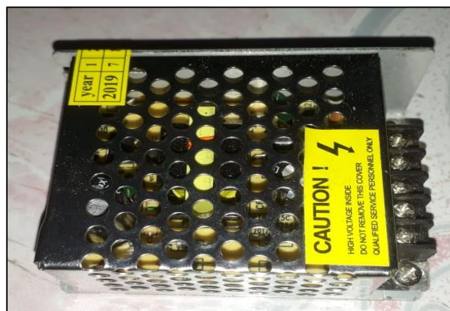
Gambar 2.11 Switch-Mode Power Supply 12V 3.2A
