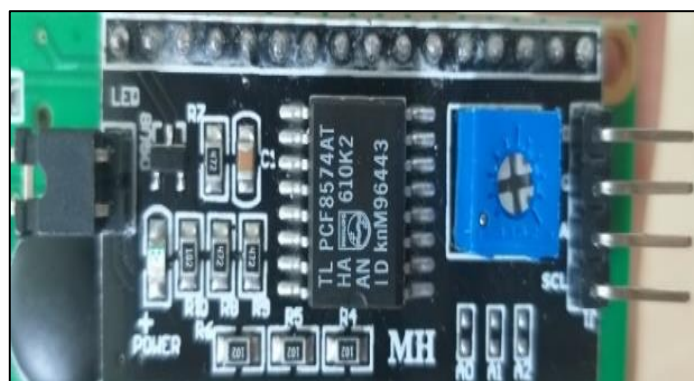
Gambar 2.9 Modul I2C ( Inter Intergrated Circuit )
