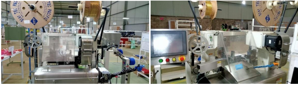
Gambar 1.3 Autocutting Crimping dan Stripping
