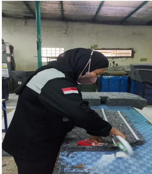
Gambar 2. 16 Proses Assy Double Tape
