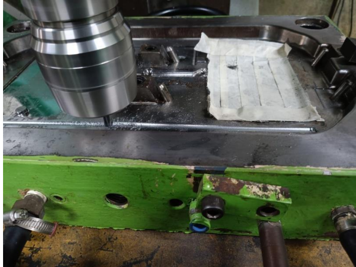
Gambar 2. 1 Contoh Proses Repair Mold
