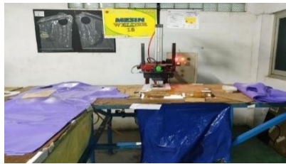
Gambar 2. 12 Proses Welder Service Hole
