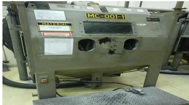
Gambar 2.11 Panel On-Off Mesin Blasting
