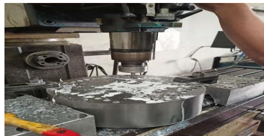
Gambar 2.4 Pengeboran Stainless Steel
