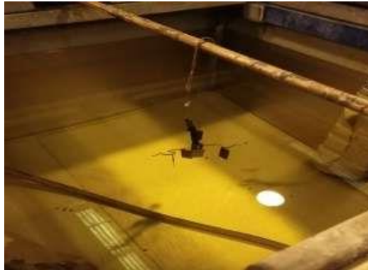
Gambar 2.17 Proses Pelapisan Kadium
