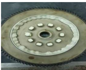
Gambar 2.5 Proses Masking Turbin Disk
