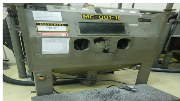
Gambar 2.11 Panel On-Off Mesin Blasting
