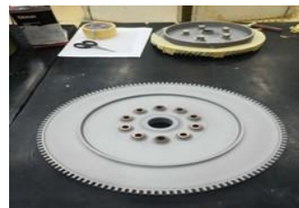
Gambar 2.6 Proses Blasting Turbin Disk
