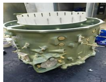
Gambar 2.8 Proses Masking Air Intake Casing
