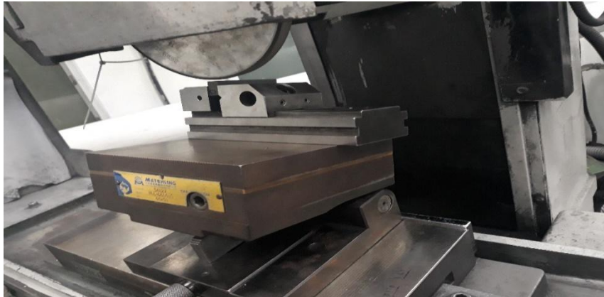
Gambar 6. Proses Grinding Punch
