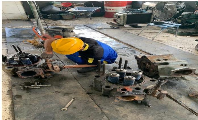
Gambar 2.7 perbaikan cylinder head Nigata
