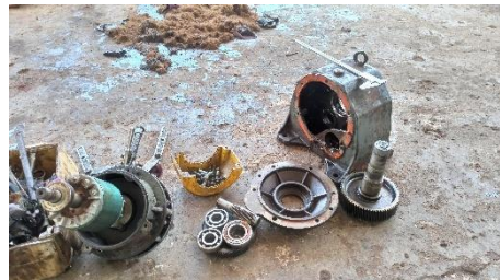
Gambar 2.4 Proses Penggantian Bearing
