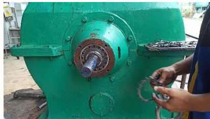
Gambar 2.4 Proses Penggantian Bearing
