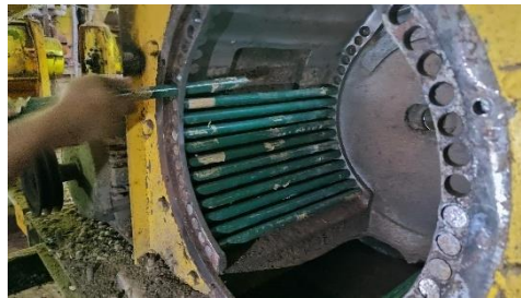
Gambar 2.5 Pergantian As bar Rotor Rod Ripple Mill
