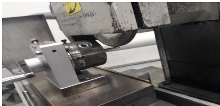
Gambar 2. 16 Proses Grinding Punch Hole
