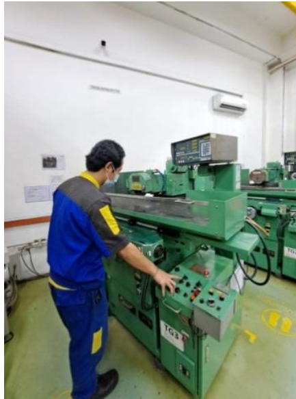
Gambar 2. 1 Proses sharpen mata potong tooling
