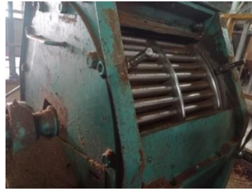
Gambar 2.2. Bagian as pemecah biji sawit(Ripple Mill)
