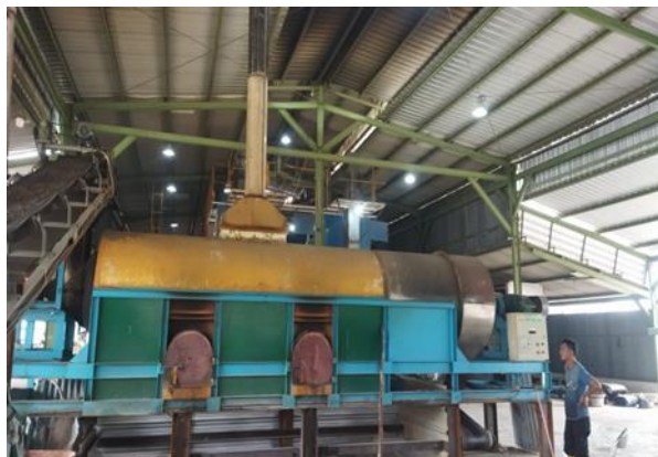
Gambar 2. 7 RD (Rotary Dryer) bahan bakar kayu api
