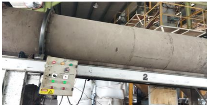
Gambar 2. 6 RD (Rotary Dryer) Bahan bakar solar
