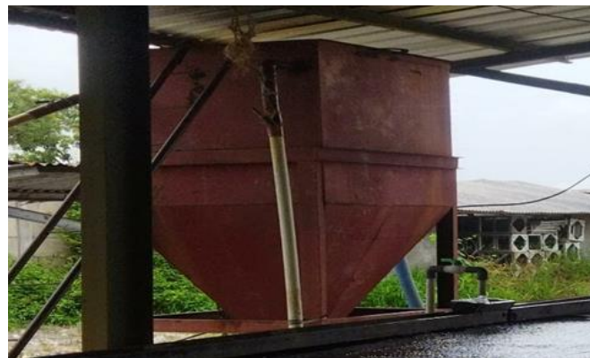
Gambar 2. 3 Hopper hasil olahan shaking table kiri
