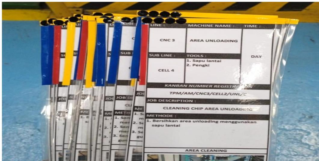
Gambar 2.3 : Kanban Autonomous Maintenance
