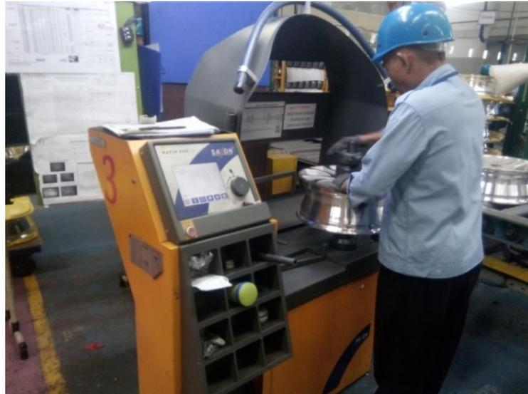
Gambar 2.31 : Proses Balancing
