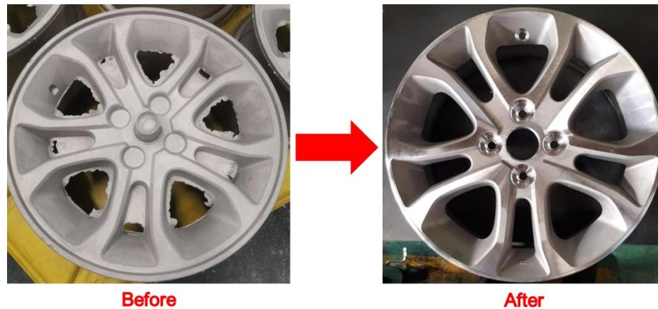
Gambar 2.23 : Hasil Proses Lini Machining
