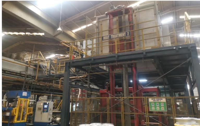
Gambar 2.21 : Proses Heat Treatment
