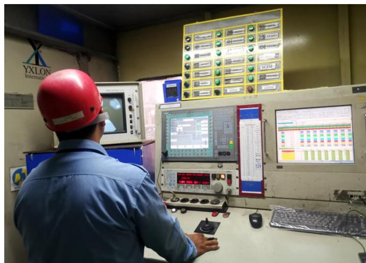
Gambar 2.20 : Proses X-Ray Inspection
