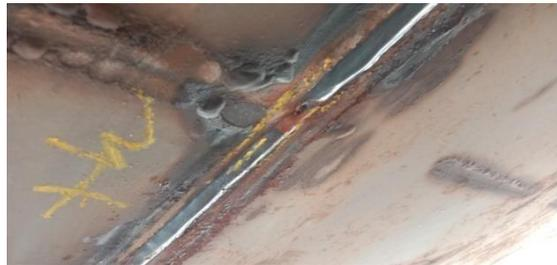
Gambar 2.3 Inspeksi *Visual weld join plate*
