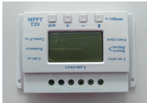
Gambar 2.6 Maximum Power Point Tracking
