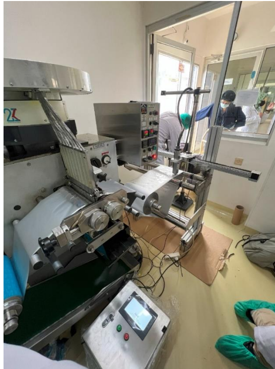
Gambar 2.5 Dokumentasi Trial Moving Head System di PT. Lloyd Pharma Indonesia untuk Printing Expired Date
