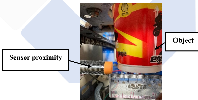
Gambar 4. 3 Percobaan Sensor Proximity
