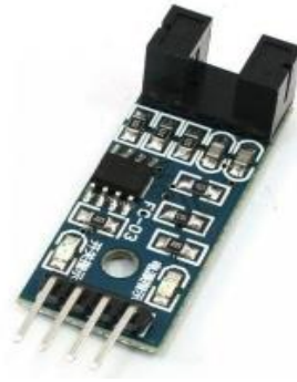
Gambar 4.6 Sensor Rotary Encoder FC-03 [8]
