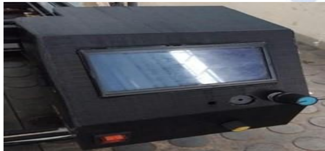
Gambar 4. 9 box control ramps 1.4
