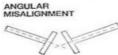
Gambar 2. 1 Angular misalignment (Swandono, 2019)
