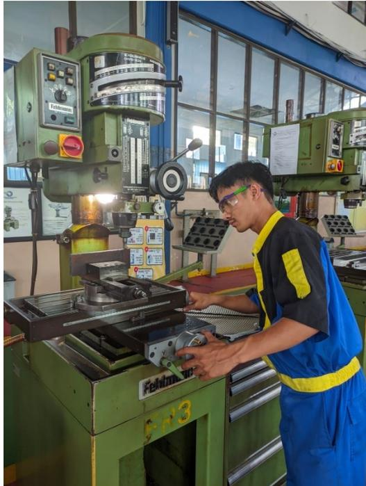
Gambar 4. 5 Proses frais *braket caliper 1*
