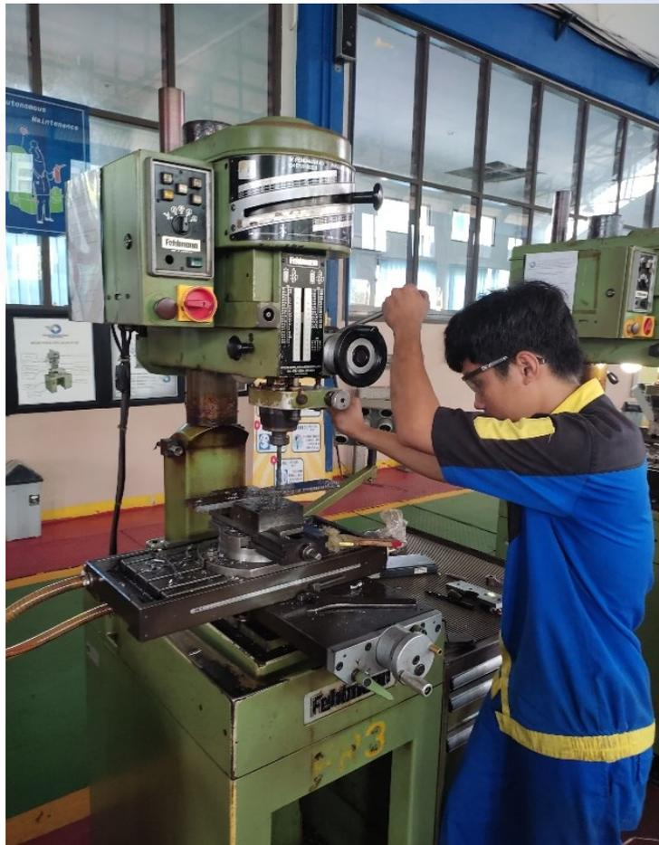
Gambar 4. 7 Proses frais *braket caliper 2*
