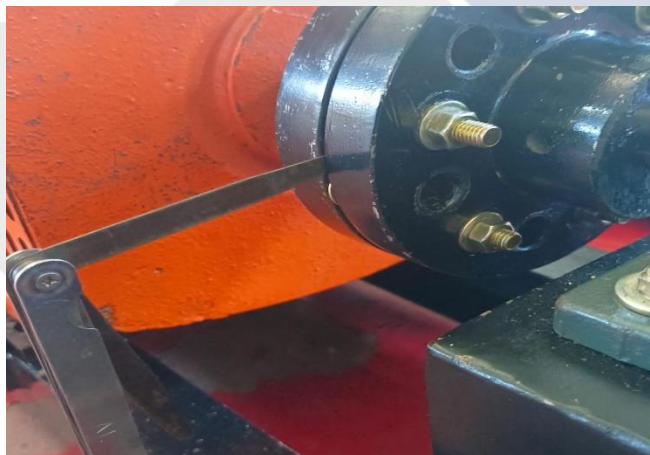
Gambar 3. 13 Angular Misalignment Posisi Horizontal
