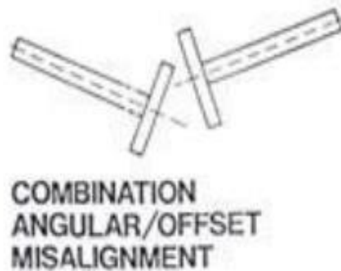
Gambar 2. 12 Combination Angular/Offset Misalignment
