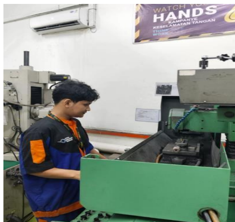
Gambar 2. 1 Proses Sharpen mata potong Tooling
