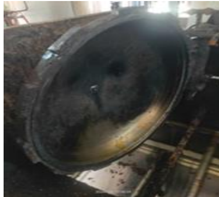
Gambar 2. 2 Penggantian Paking Bottom Clutch Door Sterilizer
