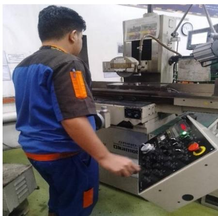
**Gambar 2. 1** Proses Sharpen mata potong Tooling
