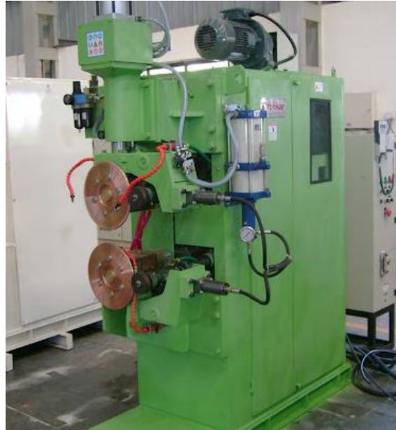
Gambar 2. 2 Seam Fuel tank
