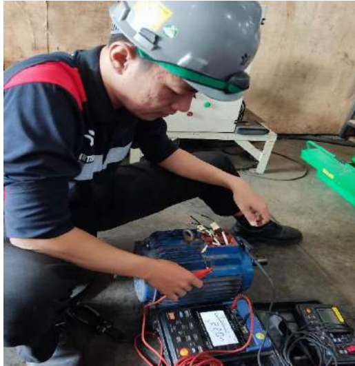
Gambar 2.4 Proses Resistance Test
