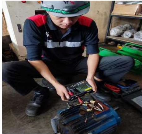
Gambar 2.3 Proses Resistance Test
