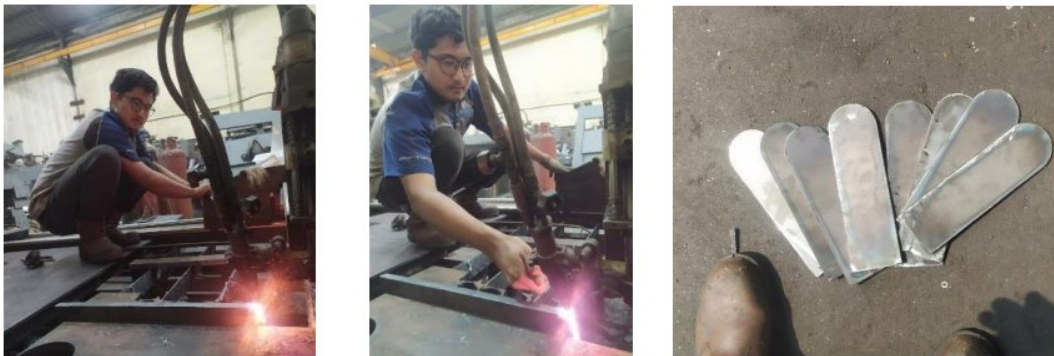
Gambar 2.1 Pengoprasian Mesin CNC Plasma Cutting
