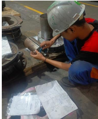
Gambar 2.5 Proses Pungukuran Micrometer
