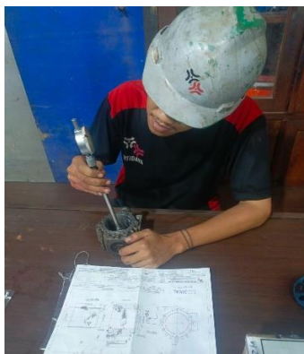
Gambar 2.4 Proses Pengukuran Bore Gauge
