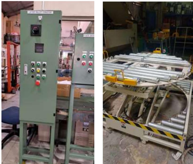
Gambar 1. 10 *Lifter Pallet Conveyor*
