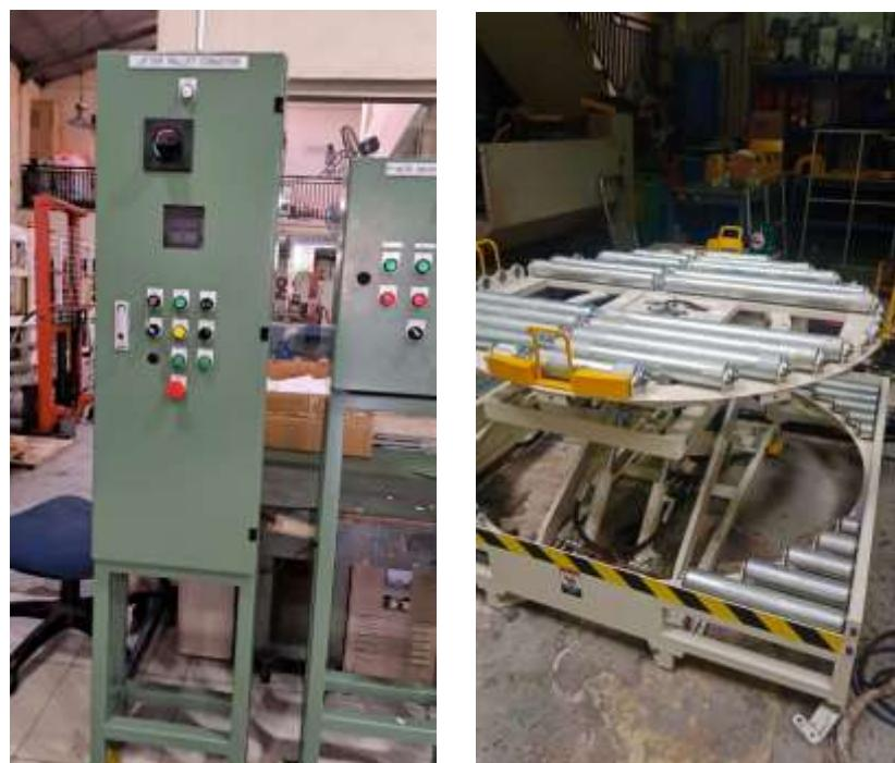
Gambar 1. 10 *Lifter Pallet Conveyor*
