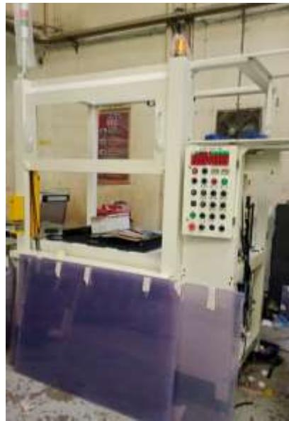
Gambar 1. 6 *Leak test machine*
