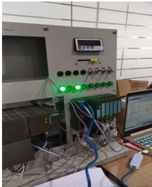
Gambar 2. 2 Training Software Tia Portal V16 dan PLC siemens
