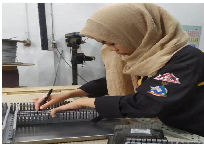
Gambar 2. 22 Pengukuran Duct Kabel PLC Panel Weighing Table
